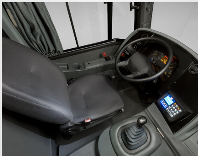
Asiento del conductor ergonómico y con panel multiplex Ergonomic driver's seat with multiplex panel
